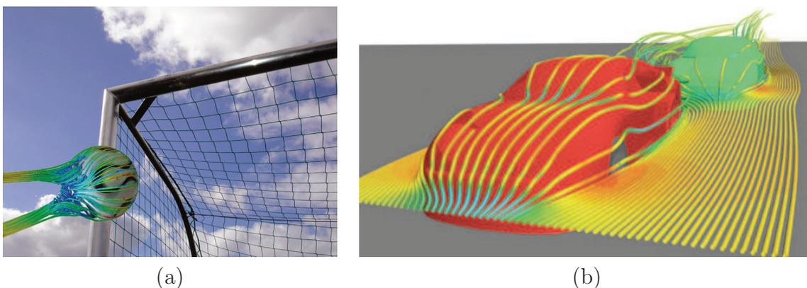
Figure 1: CFD studies aerodynamics in sports. In (a), CFD research predicts the flight of a soccer ball. In (b), a simulation of two NASCAR cars visualizes the streamlines of air produced as a car drafts and is about to pass another.
