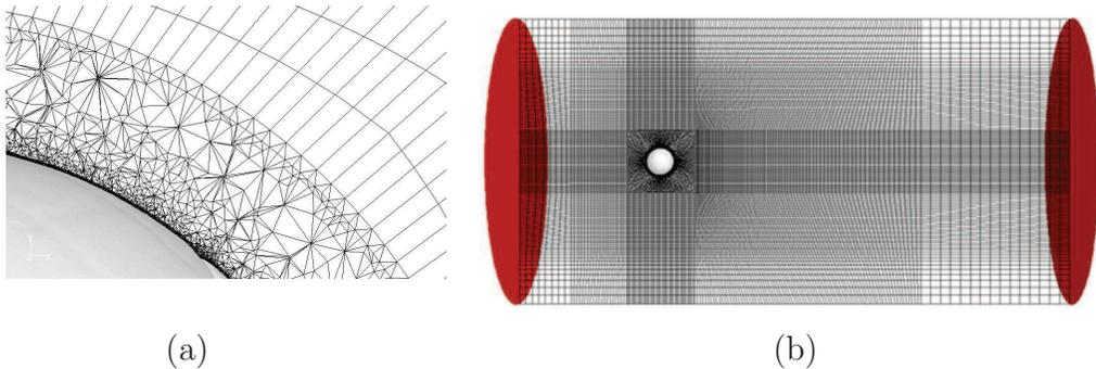
Figure 2: An important step in CFD simulations is capturing the geometry of a soccer ball with a 3D non-contact laser scanner. The mesh in (a) has approximately 9 million cells. As seen in (b), the space around the ball is meshed as to determine the flow of air.
